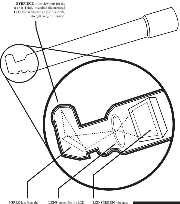
MIRROR reflects the magnified LCD screen to the viewer's eye piece
